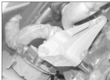
23.20b Engine/transmission right-hand mounting
