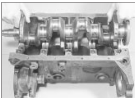
20.15 Fitting the crankshaft
