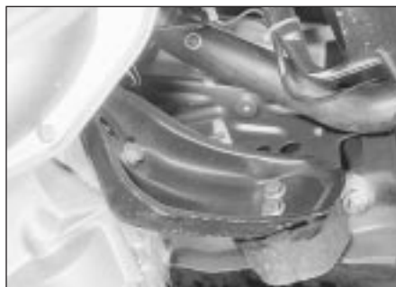
23.20a Engine/transmission left-hand mounting
